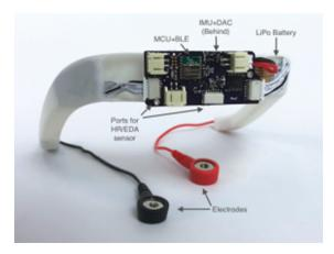
Fig. 1. Electrodes attached behind the ear are used to transmit a small electrical current to the vestibular system, providing proprioceptive information to the user.
