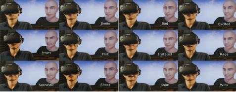
Fig. 4. (top) The Fascia device, a smart sleep mask that collects EEG, EOG, EMG, heart rate, head movement and skin temperature. (bottom) The user's real-time expression and emotion are mapped into the user's VR avatar.
